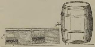
the top of the trough, and the end of the trough is furnished with a cock inserted a few inches above the level of the sand. At the other end a barrel is placed, also supplied with a cock. The whole arrangement is shown in Fig. 12.
